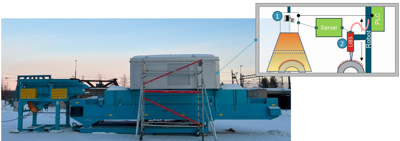
Fig.1: Test line for training and evaluation of sensor systems for heavy scrap
